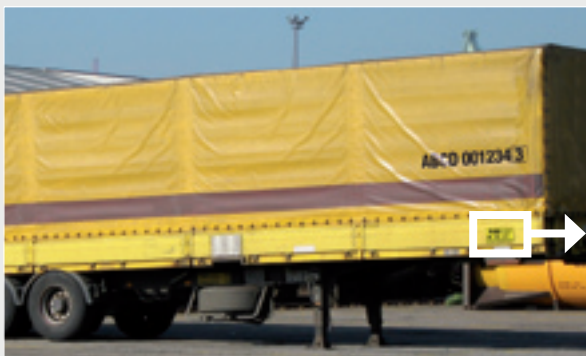
► New codification plates compliant with the EN 13044 standard for swap-bodies and semi-trailers (for each and according to preference: horizontal or vertical)
